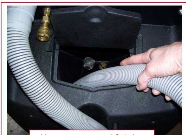
Vacuum water out of Solution Tank
